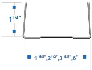
This non-structural framing member is designed to be placed on top and bottom to secure wall studs to form a lightweight structure.
